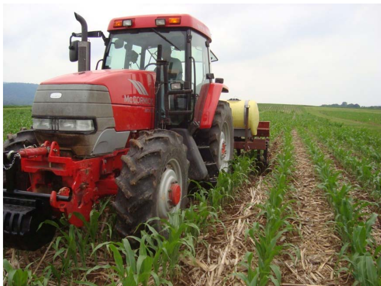
Figure 1. Interseeding no-till corn while sidedressing and applying a postemergent herbicide with the new interseeder and applicator developed at Penn State.
